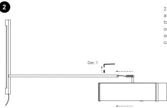
2 - Push the shade into the open end of the arm of the fixture. To do this you will first need to remove the cable trap screw (Det. 1) found on the upper side of the arm above the shade so that when you put in the shade the cable can go into the arm.
