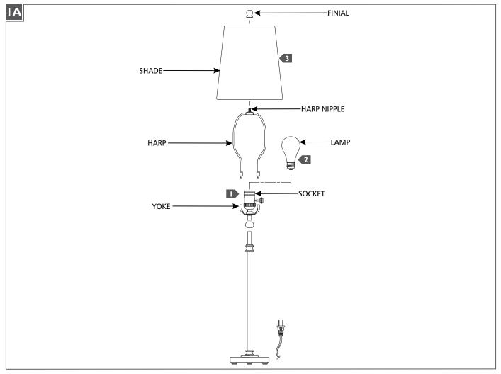
Install the harp by inserting it in the yoke.
