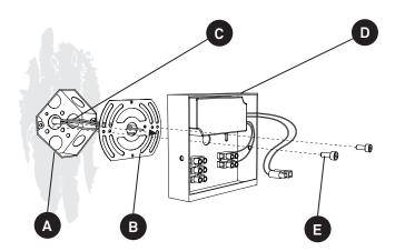
2. Feed the electrical wires (C) in through the back plate (B) and the structure (D). Fix it to the junction box (A) with the screws (E) and connect the electrical wires to the mains.
