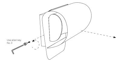
1. Remove these screws to separate the shade from the back plate.
