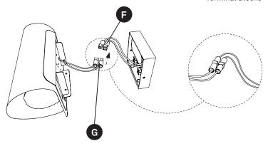
4. Take the connector from the Driver (F) and connect it to the shade connector (G).
