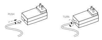
1. Plug-in led driver assembling.
