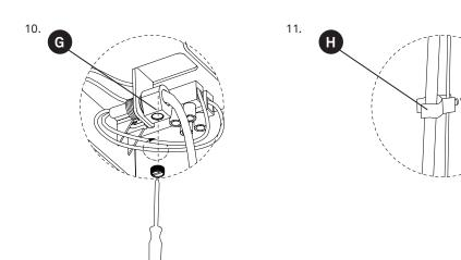
${\bf 10}.$  Tighten the screw on the electrical cable trap (G).
