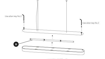
${\bf 5.}$  Fix the cover with the led modules to the fixtures. Don't touch the led modules.
