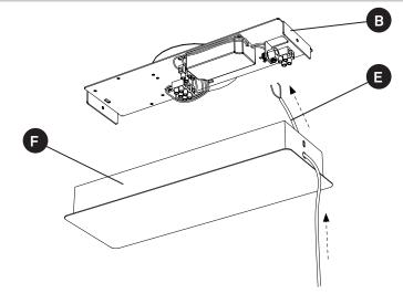
**8.** Now take the 2 cables coming from the lamp (E), and feed them through the canopy cover (F) and make the connections to the driver in the canopy (B) as indicated at point 9.
