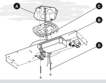
**6.** Feed the electrical wires (C) in through the electrical back plate (B), fix back plate to the junction box (A) with the screws and spherical nuts (D) and prepare to wire up the driver.
