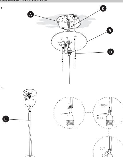
**1.** The canopy is made up of a back plate with the electrical connections on it and a semi spherical cover.
