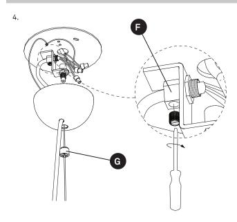
4. Tighten the screw on the electrical cable trap (F). Once all your wiring is complete raise the
