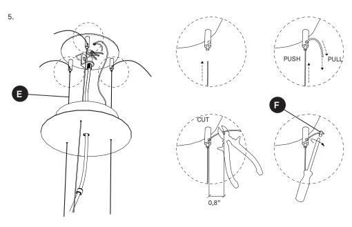
5. Adjust the height of your lamp by raising or lowering the stainless steel adjustment cable (E) and cut off the excess. For added security put on the stopper (F) and tighten it.
