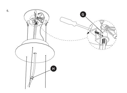
6. Tighten the screw on the electrical cable trap (G).
