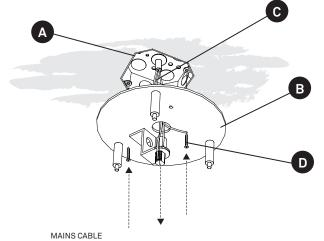
1. The canopy is made up of a back plate with the electrical connections on it and a front cover.
