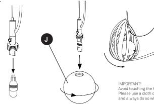
Avoid touching the halogen lamp with your fingers at all times. Please use a cloth or tissue paper when handling the bulb, and always do so when the bulb is cold.
