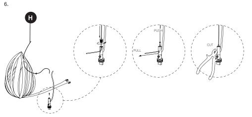
**6.** Push the steel cable (H) into the nipple of the suspension system. Adjust the height of your lamp by raising or lowering the stainless steel adjustment cable and cut off the excess.
