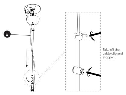
2. Adjust the height of your lamp by raising or lowering the electrical cable (E). Undo the steel cable and take off the cable clip and the stopper.
