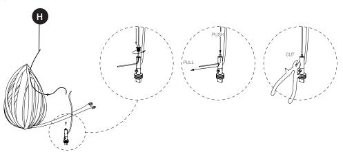
**6.** Push the steel cable (H) into the nipple of the suspension system. Adjust the height of your lamp by raising or lowering the stainless steel adjustment cable and cut off the excess.
