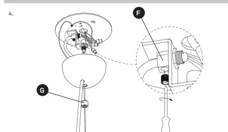
**4.** Tighten the screw on the electrical cable trap (F).
