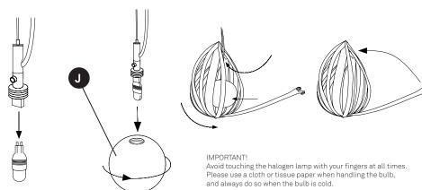
8. Plug in the G9 lightbulb. Insert the G9 light bulb holder and screw the glass ball (J) onto it.
