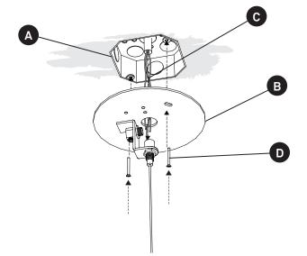
1. The canopy is made up of a back plate with the electrical connections on it and a semi spherical cover.
