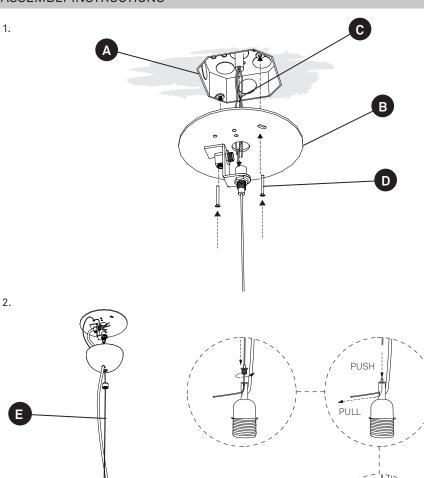
**1.** The canopy is made up of a back plate with the electrical connections on it and a semi spherical cover.
