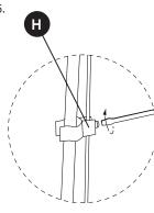
4. Tighten the screw on the electrical cable trap (F).
