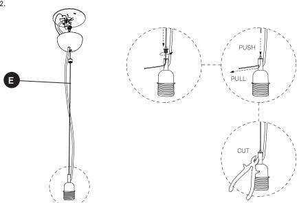
2. Adjust the height of your lamp by raising or lowering the stainless steel adjustment cable (E) and cut off the excess.
