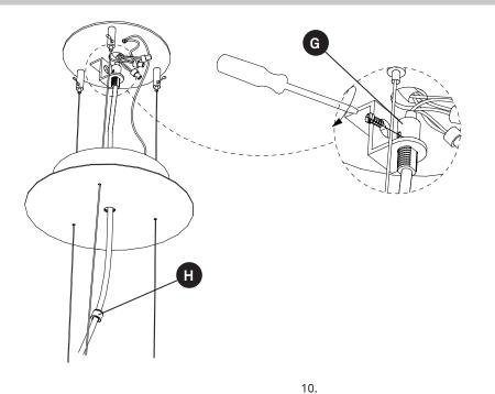
8. Tighten the screw on the electrical cable trap (G).
