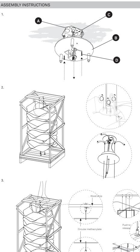
1. The canopy is made up of a back plate with the electrical connections on it and a front cover.
