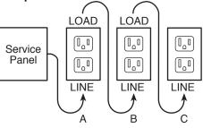
Placing the GFCI in position A will also provide protection to "load side" outlets B and C. On the other hand, placing the GFCI in position C will not provide protection to outlets A or B. Remember that outlets A, B, and C can be in different rooms.
