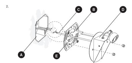
2. Feed the electrical wires (C) through the back plate (B) and the structure (D) and connect the electrical wires to the main.
