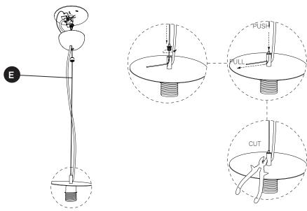
2. Adjust the height of your lamp by raising or lowering the stainless steel adjustment cable (E) and cut off the excess.
