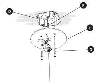
**4.** The canopy is made up of a back plate with the electrical connections on it and a semi spherical cover.
