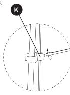
7. Tighten the screw on the electrical cable trap (I).
