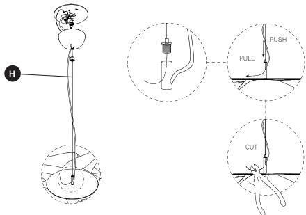
**5.** Adjust the height of your lamp by raising or lowering the stainless steel adjustment cable (H) and cut off the excess.
