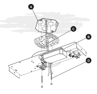
**5.** Feed the electrical wires (C) in through the electrical back plate (B), fix back plate to the junction box (A) with the screws and spherical nuts (D) and prepare to wire up the driver. Use Allen key No.2,5 to do it.
