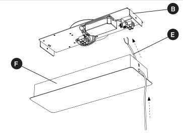
7. Now take the 2 cables coming from the lamp (E), and feed them through the canopy cover (F) and make the connections to the driver in the canopy (B) as indicated at point 9.
