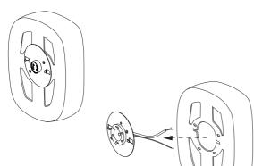
Remove the electrical back plate by detaching it from the shade.
