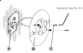
Fix the electrical back plate (B) to the junction box (A) with the screws (C).
