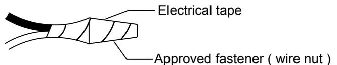
7. Connect the black fixture lead to the black wire in the outlet box. Fasten the joined wires as in step 6.
