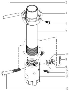
6) Route the Coupling cover (6), Canopy Ring (5), Canopy (4) and Hanger Ball (3) through the Downrod (7) in turn, and then install the Lock pin (2) through the hole on the Downrod (7). Slip the hanger ball (3) upward to lock Pin (2), and fix it by Screw (1), then slip down the Coupling Cover (6) in correct position.
