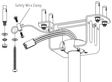
5) Connect the wire connector plugs correctly. The wire connector plugs design with fool proof device, please don't force to plug. Otherwise it may affect the normal use of the light fan or burn the fan motor.
