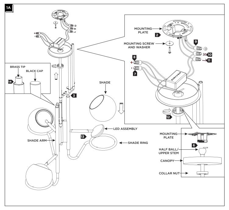
1 Remove the mounting plate and driver from the canopy.
