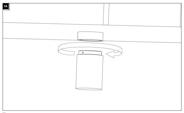
**16** Install the shade by screwing into the shade base. Repeat for remaining shades.
