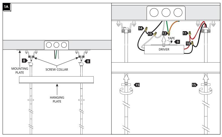
8 Insert the half ball/stem assemblies through the hanging plate and slide the half ball into the screw collars.
