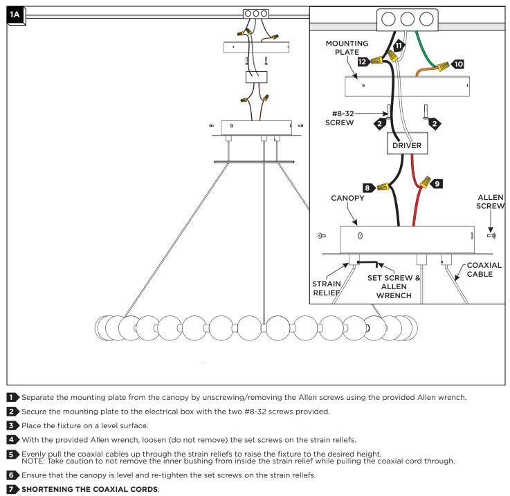
A If shortening of the coaxial cords is necessary, take note of the wire connections from the coaxial cables to the driver and remove the wire nuts.
