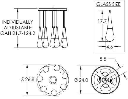
Mounting Method: Mounts to Building Structure
