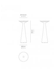
Dama pro is a battery-operated portable and rechargeable table lamp. It is equipped with: contact charging base, dimmer touch control and a light colour temperature selection function, 2700 or 3000K (dynamic white). Available also with a USB-a port for charging mobile devices.
