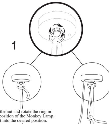
Slightly unscrew the nut and rotate the ring in order to adjust the position of the Monkey Lamp.
