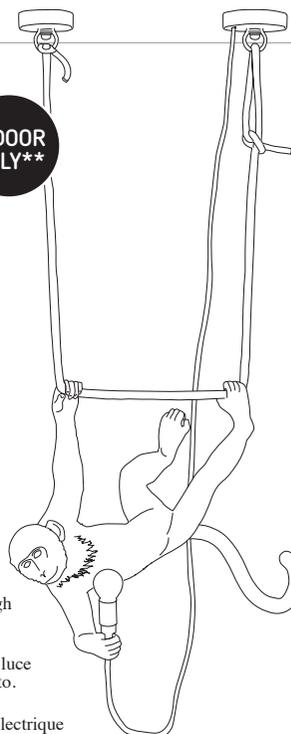
Cut the cord in order to get it through the hole on the ceiling hook.
