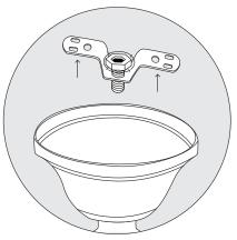
**1.** Unscrew the bracket from the semi-sphere
