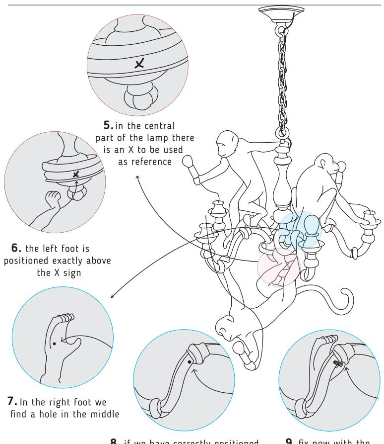
8. if we have correctly positioned the right foot, the hole of the left hand will match perfectly with the hole on the chandelier arm
