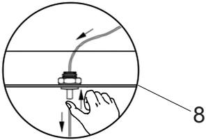
**Note:** Press the wire restraint to adjust the desired length of cable.
