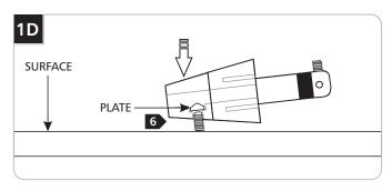
Tap the conical connector on a hard surface with the set screw facing down, so the plate inside drops into place.
