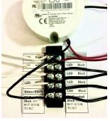
NOTE: The **Grey** and **Purple** wires are used for 0-10V dimming. If not applicable cap wires. Wires must be capped separately, or pendant will dim to zero.
