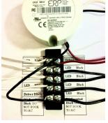
NOTE: The Grev and Purple wires are used for 0-10V dimming. If not applicable cap wires. Wires must be capped separately, or pendant will dim to zero.
