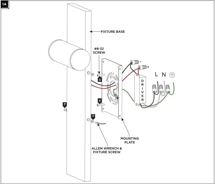
1 Connect the fixture to a suitable ground in accordance with local electrical codes.
