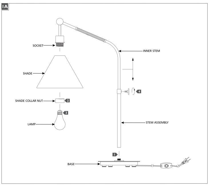
**I** Screw the stem assembly to the base.
