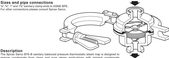
The Spirax Sarco BT6-B sanitary balanced pressure thermostatic steam trap is designed to remove condensate from clean and pure steam applications with minimal condensate retention. Applications include sterile steam barriers, block and bleed installations, mains drainage and CIP/SIP of vessels and reactors and process lines. Manufactured in 316L, the crevice free body design of the BT6-B incorporates a 15° angled seat to ensure full drainability.
