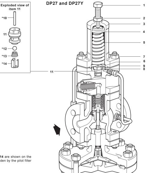
\* **Note:** Items **10**, **12**, **13** and **14** are shown on the exploded view, as they are hidden by the pilot filter on the main illustration.
