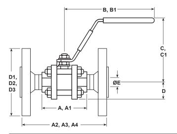
A : Screwed and Butt weld
