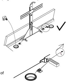
If optical socket is on rear LH side of TV, draw the loose lead out of the port and lay across TV Lift cover board as shown. Use cable clip (R) on each side to keep leads straight and out of harms way.
