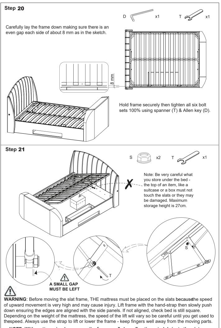
NOTE: With mattress in place, move the frame up & down five times to lubricate the pistons.
