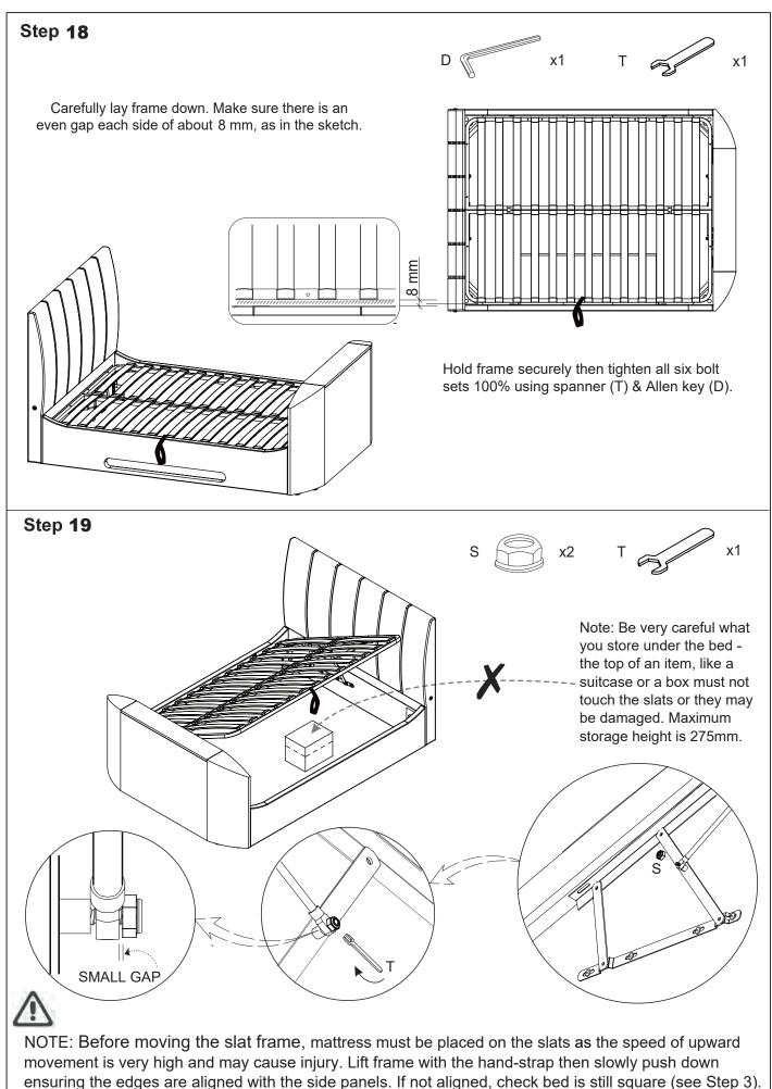
Depending on the weight of the mattress, the speed of the lift will vary so be careful until you get used to the speed. Always use the strap to lift or lower the frame - keep fingers well away from the moving parts.
