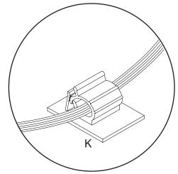
Keep wires tight - peel off cover from cable clips & adhere to back of TV.
