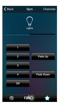
A room to control curtains and blinds will have "Open", "Stop" and "Close" options whereas a lighting room will have a number of scene buttons, fade up, fade down and off (both displayed above).
