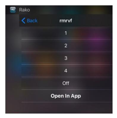
If the Rako App is running in the background a section headed "Rako" will contain the room list. Select a room to open a simplified wall plate screen. From here lights can be controlled as if from a keypad, it is not possible to set scenes or control individual channels.
