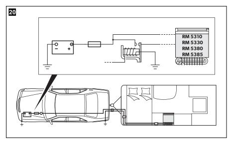
Run the cable to the heating element (connections 3 and 4) via a relay controlled by an ignition socket to prevent the vehicle battery from completely discharging if the engine is switched off accidentally (fig. 20).
