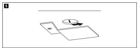
Shield the end of the opening with a deflector to prevent sludge or dirt from getting inside while driving (fig. 5).
