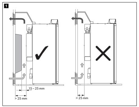
The distance between the refrigerator and the rear wall must be min. 15 mm – max. 25 mm (fig. 2), page 9).
