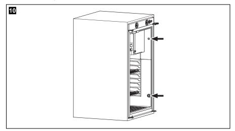
► Fasten the four screws through the four plastic washers in the sides of the refrigerator (fig. 10), and further into the wall.
