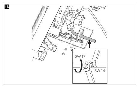
Connect the refrigerator to the gas supply securely and without any voltage according to fig.
