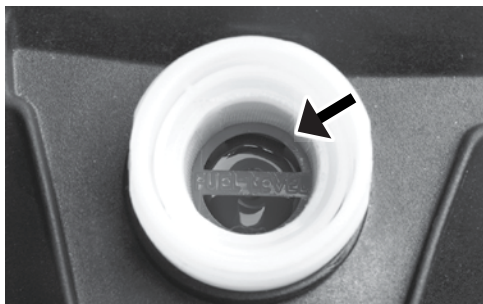
(Fig. 4) Maximum Fuel Fill Level
