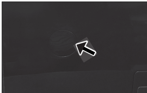
Fig. 28 Fuel Drain Access Cover
