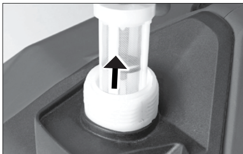
Figure 18 – Removing the Fuel Strainer
