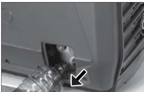
(Fig. 14) – Draining Engine Oil
