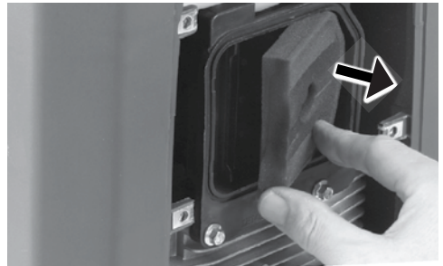
Figure 17 – Removing the Air Filter Element
