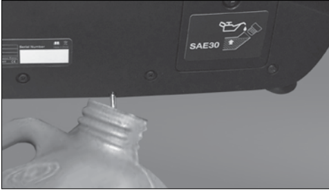
Figure 29 – Collecting Drained Fuel
