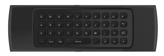
The keyboard composed by the 38 keys. Backspace:Delete previous character CAPS:Caps Lock ENTER:Confirm the operation SPACE:Spacebar ALT:Numeric characters switch
