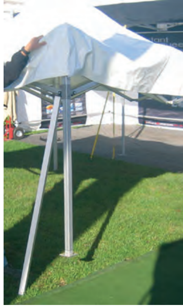
1) Lift the corner of the tent lightly and insert the rigging tool under the slider
