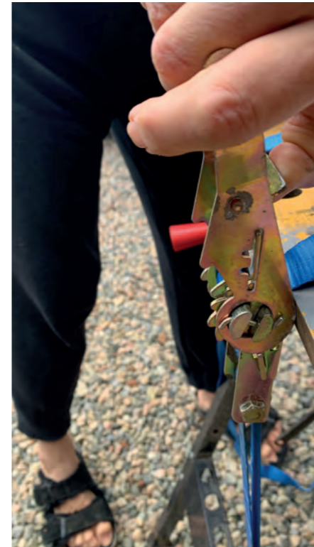
3) Whilst holding the detente down, open out the buckle 180° to unlock the ratchet, then ease the buckle along the long part of the strap to the end
