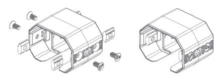
$\odot$  7. ASSEMBLE TUBE PLATES TO TUBES AND TIGHTEN TO 5Nm
