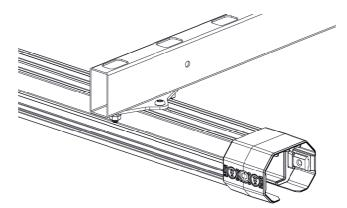
$\textcircledightarrow$  10. INSTALL MARKING PLATE AND INSERT TROLLEYS (REFER TO P15 OF SPACERAIL HOOK INSTRUCTIONS). INSERT END CAPS AND TUBE PLUGS.
