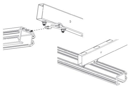
**Note:** Ensure Rail is level, parallel with any surrounding objects and not bent, twisted or distorted from the installation process. Check using a spirit level and adjust as necessary.
