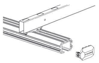
→ Insert Trolleys in to Rail (see separate instructions) and ensure they run freely and smooth the whole length of the Rail. Repeat process for second End cap.
