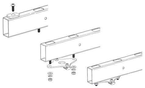
$\ominus$  8. INSTALL RAIL TO TUBE PLATES. TIGHTEN TO 5Nm
