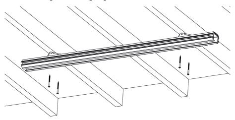
**Note:** Ensure Rail is level, parallel with any surrounding objects and not bent, twisted or distorted from the installation process. Check using a spirit level. You may need to add shims or packing pieces under the Ceiling Plates to get correct alignment.
