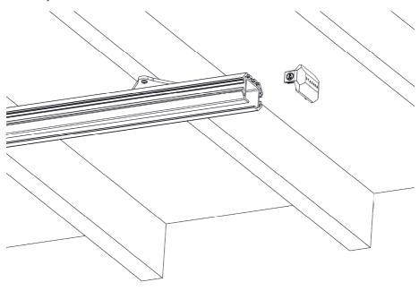
→ Insert Trolleys in to Rail (see separate instructions) and ensure they run freely and smooth the whole length of the Rail. Repeat process for second End cap.
