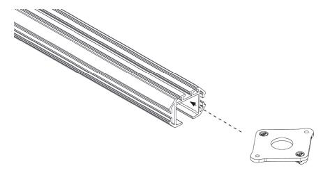
$\rightarrow$  Slide Ceiling Plate to positions marked earlier and tighten to 7Nm with 4mm Hex Key.
