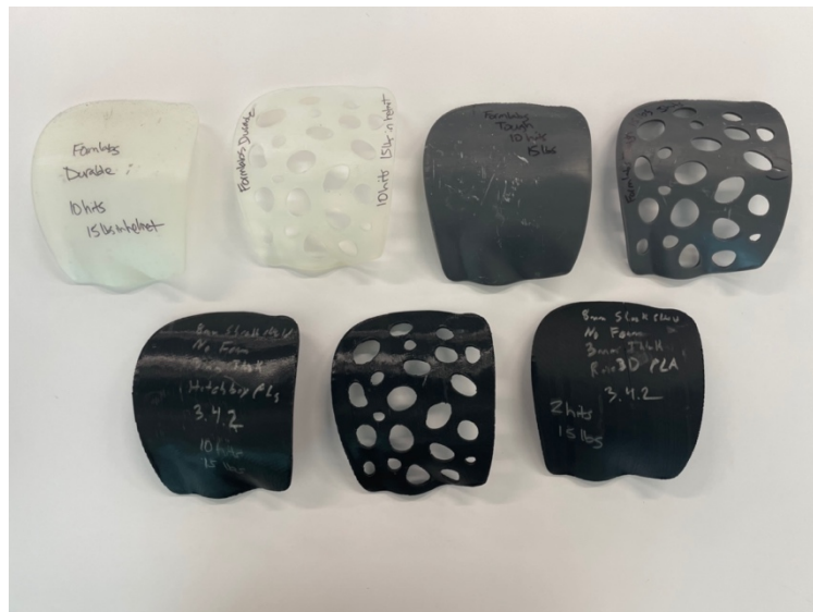
Figure 1. Testing Guards (Top Row L-R: Formlabs® Durable resin, solid; Formlabs® Durable resin, holed; Formlabs® Tough resin, solid; Formlabs® Tough resin, holed; Bottom Row L-R: Hatchbox® PLA, solid; Hatchbox® PLA, holed; Raise3D® PLA, solid)
