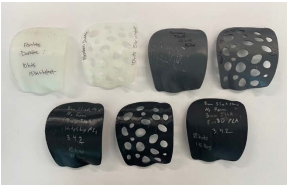
Figure 2. Shoulder Guards: (Top Row, Left to Right) Formlabs Durable Solid, Durable Holed, Tough Solid, and Tough Holed and (Bottom Row, Left to Right) Hatchbox PLA Solid, Hatchbox PLA Holed, and Raise3D PLA Solid (Source: M. Zabala and J. Larson).
