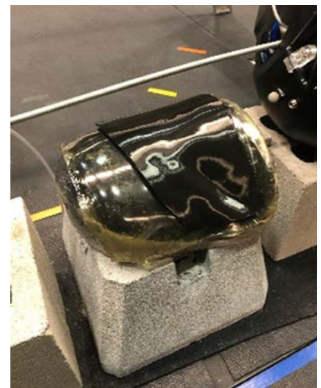
Figure 3. BOB Right Shoulder (Concrete With Overlaid ShockShield) With a Custom-Fit, 3-D-Printed Shoulder Guard (Source: M. Zabala and J. Larson).
