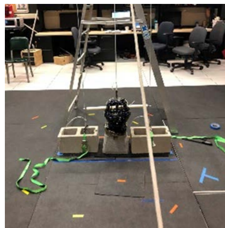
Figure 4. Setup for Impact Testing (Source: M. Zabala and J. Larson).
