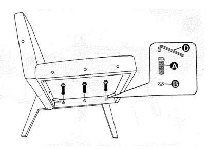
Assemble the base to one side frame. Insert the screws into the holes and tighten. Tighten to approx 90%, not too tight.
