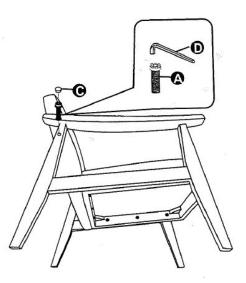
Insert the screw into the hole and tighten. Tighten to approx 90%, not too tight.
