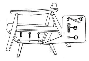
Assemble the base to second side frame. Insert the screws into the holes and tighten. Tighten to approx 90%, not too tight.
