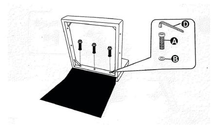
Assemble the base to the back. Insert the screws into the holes and tighten. Tighten to approx 90%, not too tight.
