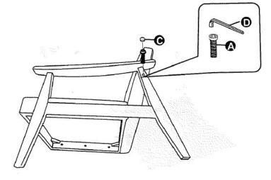
Insert the screw into the hole and tighten. Tighten to approx 90%, not too tight.
